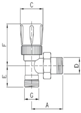
Valvola a squadra cromata termostatizzabile attacco tubo rame e plastica Angle chrome plated radiator valve with thermostatic option - connection copper and plastic pipe.
